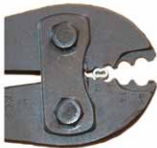
Incorrect sleeve placement
