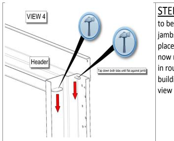
STEP 3: Use hammer to bend tabs. After jambs are locked in place by the tabs, it is now ready to be placed in rough opening on building. See view 4 and view 5.
