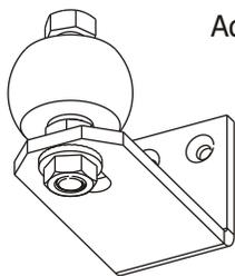
Adjust bolt on door stay so it is not protruding past flange nut.
