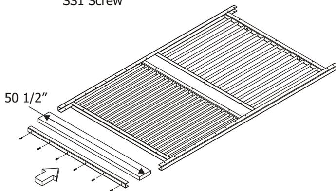
Insert a 5 1/2" x 50 1/2" (2 x 6) piece of lumber into the bottom channels.
