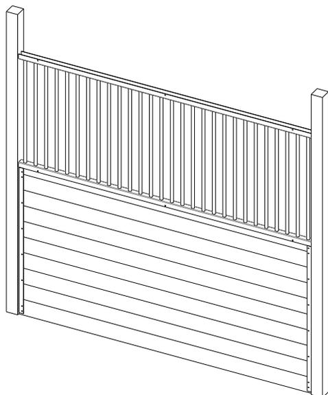
Fit the grillwork section over the last board so it rests on top of the U-channel ends.
