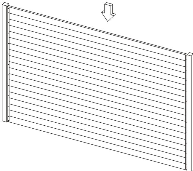
Cut lumber 1/4" to 3/8" less than the distance measured between the inside faces of the U-channel.
