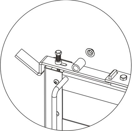
Fit long leg of lifting rod into boss of latch arm then attach lifting rod push cap onto end.
