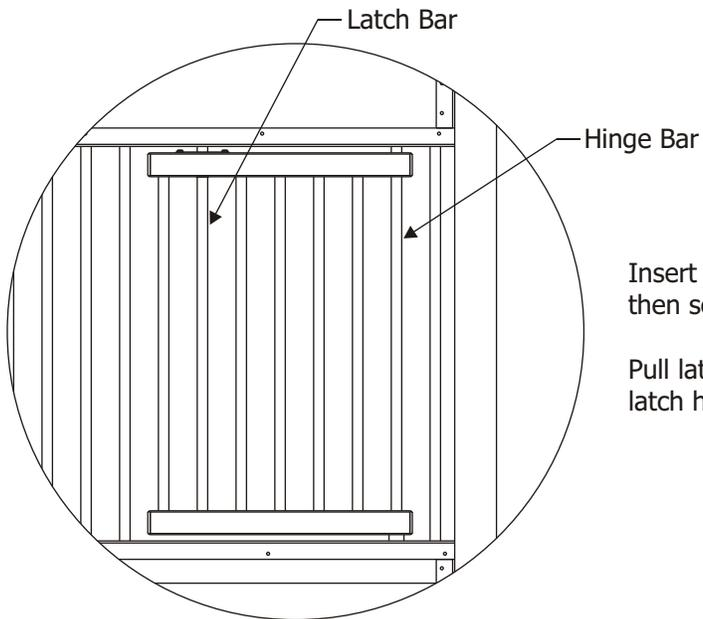
Insert top of hinge bar completely up into hole in top channel then set bottom of hinge bar down into hole in bottom channel.
