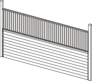
Fit the grillwork section over the last board so it rests on top of the U-channel ends.
