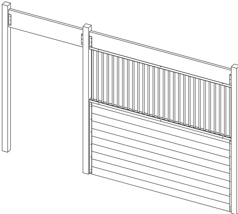
Install two 7" U-channels in the door opening aligning them with the 7" U-channels in the front.
