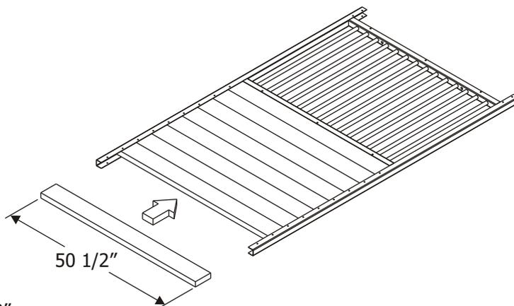
Insert bottom channel over last piece of lumber so it is flush with bottom of U-channels. Use a rubber mallet and block of wood if necessary so not to damage channel.
