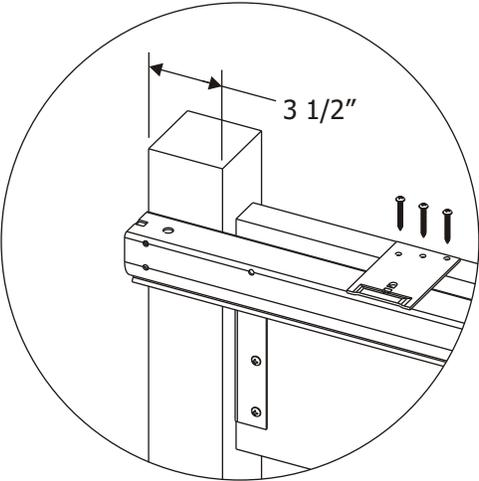
Place track with attached brackets on top of nominal 2x12 and against face of posts. Edge of track should be approximately 3 1/2" from door opening edge of post (flush with outside edge of 4x4).
