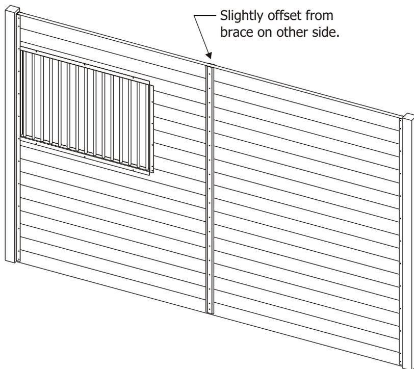
Center a 94 1/2" wall brace on the wall and fasten with SS1 screws.
