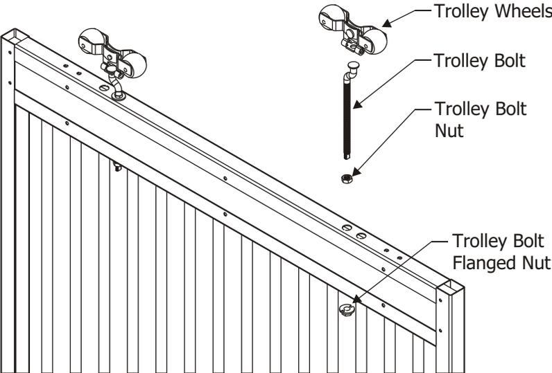
Insert trolley bolt through hole in trolley wheel assembly.
