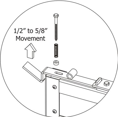
Slide latch spring over 1/4" x 3" lag then nylon washer.
