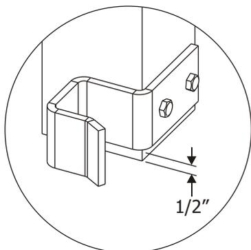
Attach post bumper to bottom of corner post approximately 1/2" above floor with provided 5/16" x 1 1/2" lags.
