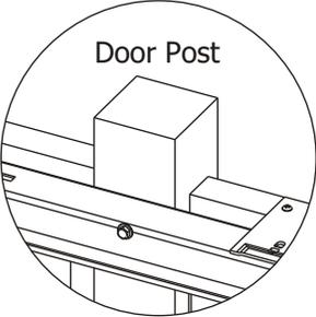
Fasten (2) 1/4" x 4" lags with washers through hole along top edge of track at door posts locations.
