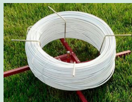
STEP 2 Use spinning jenny to lay out rail and help prevent breakage.
