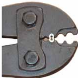
Correct sleeve placement
