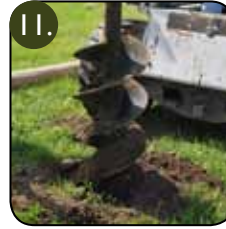
1 2" Diameter 48" Long Auger
