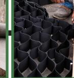
Expand panels to relax for installation. Prepare & compact subgrade to repair pre-existing ruts & support drainage. Roll out & install a water permeable barrier such as a landscape under layment. Connect & secure panels with stakes. Secure & protect your edges with a structural border. (example: pressure treated lumber) Infill Mud Management cells with crushed gravel.
