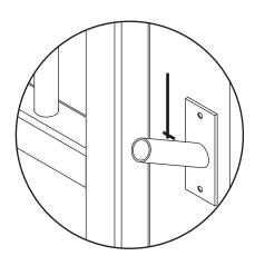
Extend centerline marks to find center of hole location.
