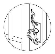
Insert pin into frame receptacle.
