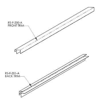
Locate 2x **RS-F-200-A** (*Front Corner Trim*) and 2x **RS-F-201-A** (*Back Corner Trim*) and mount them as shown below using the Electric drill and **HH** (*Self-Tapping Screws*).
