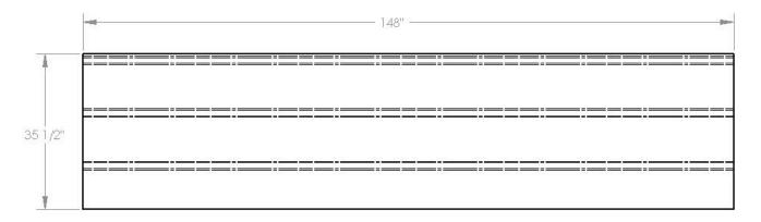
Lightly mark the *Cladding* with a pencil to indicate the position of the beams and wood for future reference. Start at one end and mount the steel using the pencil marks as a guide.
