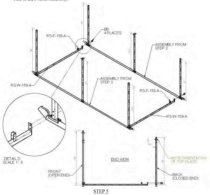
Locate 4x **RS-W-152-A** (*Mid Connector Beam*) and connect to the *Frame Assembly* previously completed in <u>Step 4</u>. Join with **BB** in 14 places as shown.
