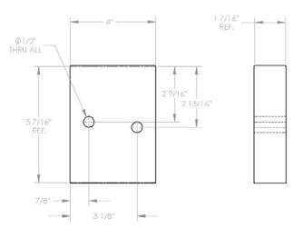
$\frac{\text{WOODEN SHIM BLOCK}}{\text{QTY} = 4x}$ - CUT 4 PIECES OF 2" x 6" LUMBER x 4" LONG - DRILL 2x 1/2" HOLES AS SHOWN IN EACH
