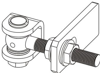
Remove nut and washer on Subassembly B.
