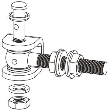
Attach hinge assembly to post hinge bracket as shown.
