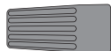
3- Properly sized wire nuts (size is based on connecting wires combined diameter)
