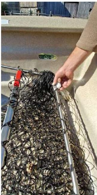
4. Recombine one of the U-bolts and plastic spacers close to one set of alignment marks on the U-rod. **Be sure not to entangle the net in the U-bolt or behind the plastic spacer.**
