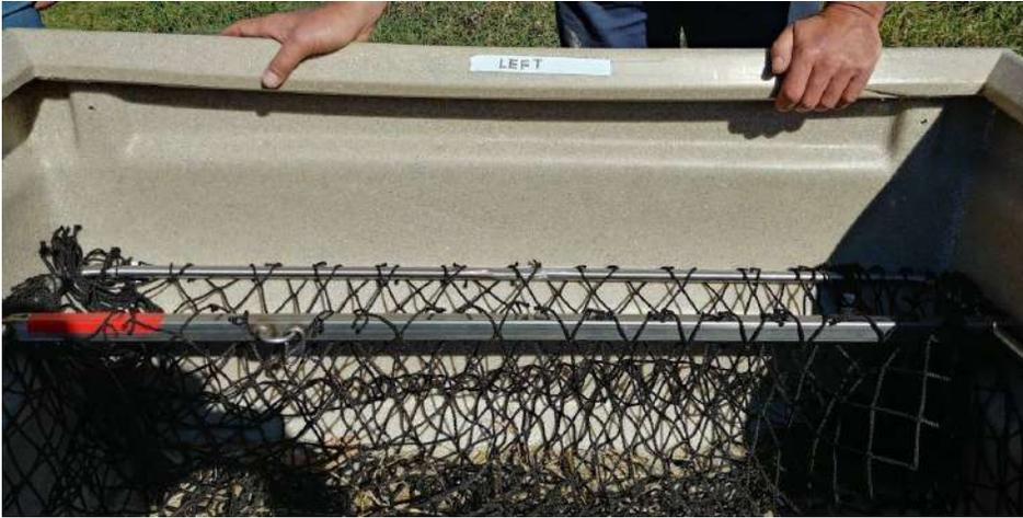
7. Lift one leg of the U-rod out of the feeder through the wide notch in the top rim and place the end of the other leg back through its mounting hole.
