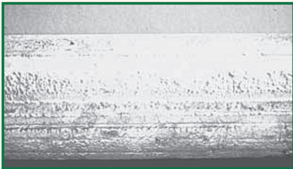
Rough coating due to phosphorous levels over 0.04% (Acceptable unless on a handrail)
