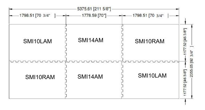
Measurements are calculated from the center of the interlocking teeth, for ease in calculating the surface area covered by several assembled mats. All measurements have an 1/8" (3 mm) tolerance.
