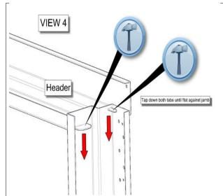
STEP 3: Use hammer to bend tabs. After jambs are locked in place by the tabs, it is now ready to be placed in rough opening on building. See view 4 and view 5.
