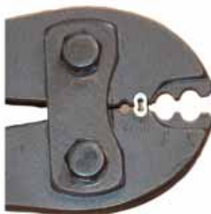
Correct sleeve placement
