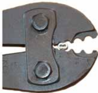
Incorrect sleeve placement
