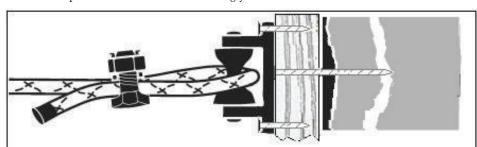
Starting at the end post, feed the leading end of the ElectroBraid™ through the insulator and secure it to itself using a copper split-bolt connector. The split-bolt should be about 2" from the end insulator. Leave at least 2" of ElectroBraid™ outside the copper split-bolt connector. Tape, cut and singe the end to prevent fraying.
