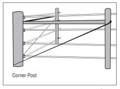
If your corner, end or gate post is large in diameter, you may want to pre-drill a hole for the spike through the post and into the end of the rail.
