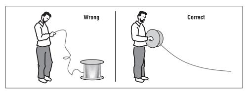
**DO NOT** take Braid<sup>TM</sup> off one end of the spool. The Braid<sup>TM</sup> will kink and could be damaged. The correct method is to unroll the Braid<sup>TM</sup> and it will not kink. (see diagram)
