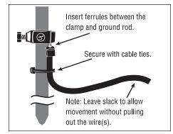
Do not confuse or combine ground rods for your house with ground rods required for an electric fence energizer. The ground rods used with a fence energizer act as receivers for electron flow.
