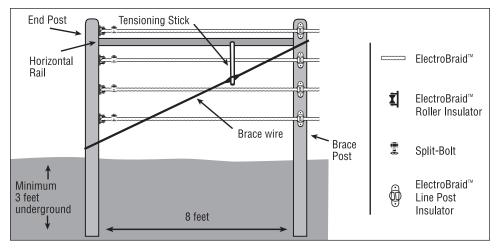
NOTE: To prevent an electrical short, make sure the brace wire and tensioning stick cannot contact any ElectroBraid<sup>TM</sup> strands
