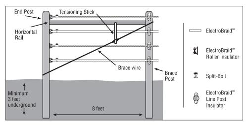
Proper Bracing will increase the effectiveness of your fence and reduce maintenance caused by post shifting. *Incorrect or insufficient bracing may lead to fence failure and may be dangerous to you and your horses.* If you are unsure of how to brace or are unsure of your soil conditions please call us at 1-888-430-3330 for assistance.
