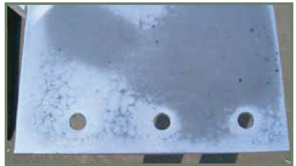
Gray coating due to temperature differences (Acceptable)
