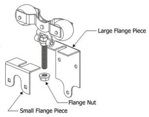
Step 7 – Align the trolley assembly over the top of the door with the 1/2" bolt going into the drilled hole.
