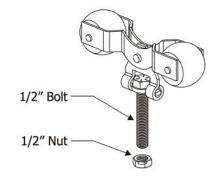
Step 5 – Slide a large and a small flange piece around the 1/2" bolt into the slots. Overlap the large flange piece on top of the small flange piece. Step 6 – Screw on the flange nut.
